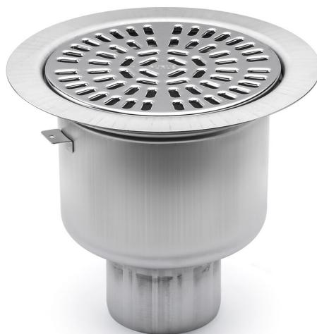
The Heavy 110 R floor drain has a 110mm bottom outlet and is for installation in concrete joists. The Heavy floor drain comes with a stainless steel water trap, clamping ring and stainless steel grate. It also comes with a protective cover that is intended to prevent any concrete or debris from installation from entering the drain.
