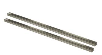
V105 Hygiene rail in stainless steel with a length of 600mm. It has pre-drilled and countersunk holes for quick wall installation. The wall rail has a smooth finish, is tight-fitting and has bevelled end pieces; making it suitable for areas where enhanced hygiene is required. The wall rail can be joined if necessary with a joining plug and is compatible with the V106 Hygiene bracket and V107 Shelf.
