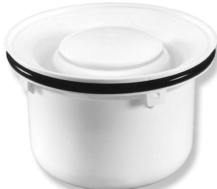
The Bolja oil barrier is manufactured in plastic and is designed for 220mm diameter floor drains without water traps. The barrier closes tightly when filled with oil. In the event of an oil spill, gaskets must be replaced. Always check with local rules and regulations for installation approval, as the Bolja functions as an oil stop, not an oil separator.
