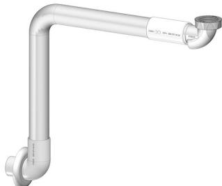
Outlet kit for wash basins with 1¼" / 1½" connections and a 40mm diameter outlet pipe. This outlet kit does not include a water trap, and is therefore compatible with Purus' PUM vertical wastes. Includes wall spacer.
