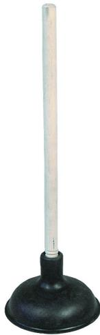
Plunger with 150mm diameter. The handle is made of wood and the suction foot in black EPDM. Used to remove blocks in, for example, wash basins, bath tubs and sinks.
