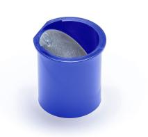
Blue plastic PUM membrane insert for vertical installation in inlets of 40mm diameter pipes. Spare part for Purus Universal Membrane products. The membrane acts as an odour barrier and is integrated within the waste, where it remains closed until opened by water flow. It is easy to clean, saves space in the installation area and has a high flow rate. Type approved by RISE.
