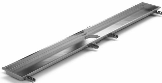
Purus channel 200 is a floor channel made of acid-resistant stainless steel for installation in concrete. The floor channel is 600×200 mm with a mid outlet and is intended for concrete flooring. The floor channel needs to be supplemented with a grating/grid depending on the environment and outlet house in plastic or acid-resistant stainless steel.
