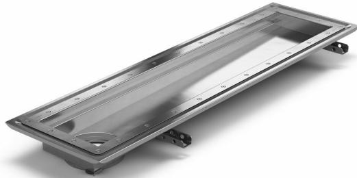
Purus channel 200 is a floor channel made of acid-resistant stainless steel for installation in concrete. The floor channel is 600×200 mm with a deep end outlet and is intended for vinyl flooring. The floor channel needs to be supplemented with a grating/grid depending on the environment and outlet house in plastic or acid-resistant stainless steel.
