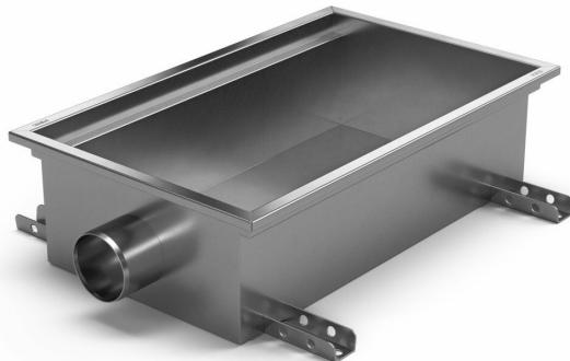
Purus channel combo is made of acid-resistant stainless steel with side outlet Ø110 mm for installation in concrete. The floor channel is 300x300x200 and is intended for concrete flooring. There is always residual water in the channel about 50 mm of water forms the water trap in the bottom of the channel and is equipped with a cleaning plug. The floor channel requires an almost continuous flow to function properly. Unsuitable in environments that set hygiene requirements.
