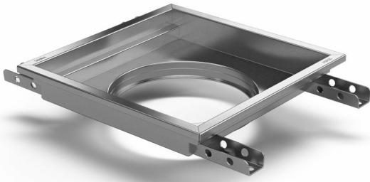
Purus channel square 200 is a floor channel made of acid-resistant stainless steel for installation in concrete flooring. The floor channel is 200×200 and is intended for concrete flooring as a surface. The floor channel needs to be supplemented with grating/grid depending on the environment and outlet house in acid-resistant stainless steel.
