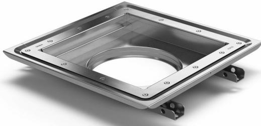
Purus channel square 200 is a floor channel made of acid-resistant stainless steel for installation in concrete flooring. The floor channel is 200×200 and is intended for vinyl flooring. The floor channel needs to be supplemented with grating/grid depending on the environment and outlet house in acid-resistant stainless steel.
