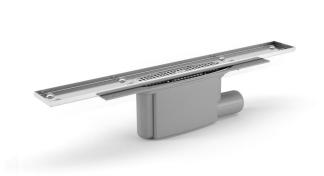
clamping ring, stainless steel frame and installation kit. It is compatible with the 800 Patterned and Limited Edition grates, which are sold separately. The NOOD water trap is a mechanical trap which closes when there is no water present, thus preventing any foul air from escaping through the drain. This linear floor drain can be installed against the wall or elsewhere in the room.
