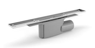
clamping ring, stainless steel frame and installation kit. It is compatible with the 800 Patterned and Limited Edition grates, which are sold separately. The NOOD water trap is a mechanical trap which closes when there is no water present, thus preventing any foul air from escaping through the drain. This linear floor drain can be installed against the wall or elsewhere in the room.
