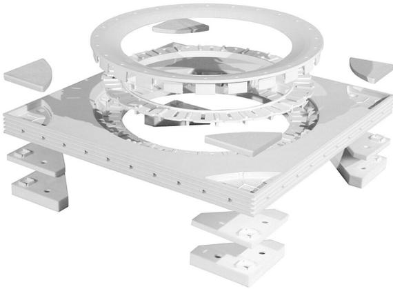
The Purus Plate 300 Multi is for installation of Purus' 130mm and 150mm diameter floor gullies into wooden joist floors. The Purus Plate is 22mm thick at the outer edge and has built-in falls to the drain. 6mm and 13mm spacer blocks can be purchased separately to increase the height. The Purus Plate 300 Multi is manufactured in ABS plastic, which can be glued.
