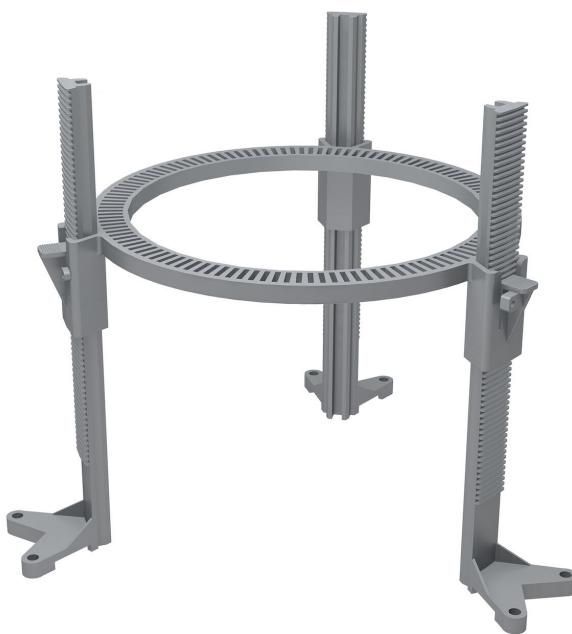
The Nordsjön Support must always be used when installing Purus floor gully into concrete floors. The Nordsjön Support secures the floor drain during installation and casting, ensuring correct installation height and scale. The Nordsjön Support meets recommended tolerance requirements for installation of floor drains +/- 4mm in height and +/- 2mm in scale according to current industry standards.
