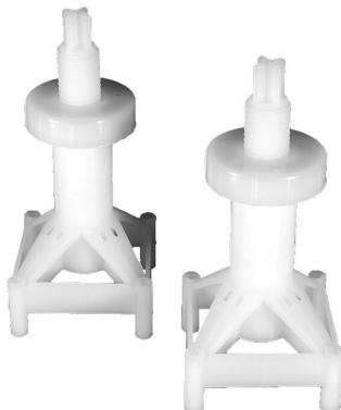
The Purus Support without top section is designed for installing Purus Line floor drains in concrete floors. The Support can be height adjusted to approximately 60mm.
