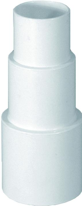
Straight reduction for pipe transition between dimension 50mm / 40/32mm in plastic. Material in ABS for gluing.
