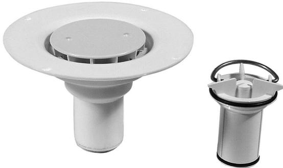
Safe Overflow for vinyl flooring has a 50mm vertical outlet and is adapted for unintentional overflow of water. The Safe Overflow for vinyl comes with a removable automatic odour stop and clamping ring. The automatic odour stop prevents any bad odours from escaping through the drainage system, even if it is dried out. The overflow must not be used as an ordinary floor drain, but can be placed underneath a sink, a kitchen ice maker or similar.
