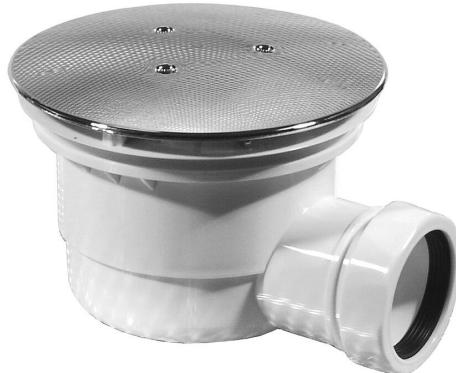
Shower tray outlet with water trap and chrome lid, designed for 90mm diameter outlet holes. It is suitable for shower trays and shower cubicles. The water trap is a mechanical odour stop designed to close when there is no water flow, thus preventing odours from escaping through the drain, even when dried out. It is therefore suitable for environments which have little or no water supply for longer periods of time. When water is flowing through, the water trap opens automatically.
