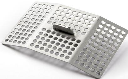
Filter basket in acid resistant stainless steel with a volume of 0.33 liters. The Filter basket is used to collect particles larger than 5 mm, e.g. leaves, so they do not fill up the water trap. The Filter basket is picked up for emptying and reassembled.
