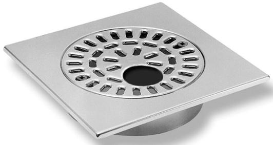
The 200x200mm stainless steel grate for tiled floors has a height of 25mm and a K3 load class (300kg), and a 40mm inlet hole. It comes with a locking device for securing to the floor. The grate consists of a square frame with a circular grate within, which can be removed for cleaning and maintenance. It is designed to fit most of Purus' floor drains with a grate diameter of 150mm.
