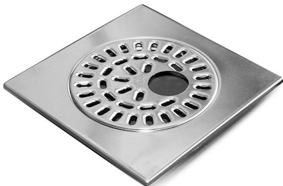
The 200x200mm stainless steel grate for tiled floors has a height of 6mm and a K3 load class (300kg), and a 40mm inlet hole. It comes with a locking device for securing to the floor. The grate consists of a square frame with a circular grate within, which can be removed for cleaning and maintenance. It is designed to fit most of Purus' floor drains with a grate diameter of 150mm.
