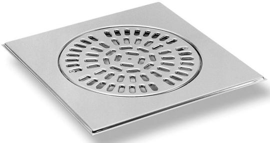
The 300x300mm stainless steel grate for tiled floors has a height of 6mm and a K3 load class (300kg). It comes with a locking device for securing to the floor. The grate consists of a square frame with a circular grate within, which can be removed for cleaning and maintenance. It is designed to fit most of Purus' floor drains with a grate diameter of 220mm.
