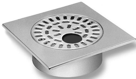
The 300x300mm stainless steel grate for tiled floors has a height of 50mm and a K3 load class (300kg), and a 50mm inlet hole. It comes with a locking device for securing to the floor. The grate consists of a square frame with a circular grate within, which can be removed for cleaning and maintenance. It is designed to fit most of Purus' floor drains with a grate diameter of 220mm.
