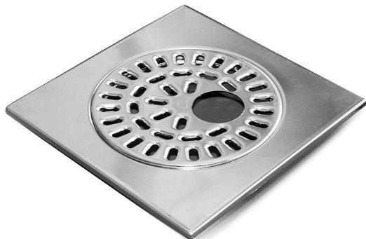
The 300x300mm stainless steel grate for tiled floors has a height of 6mm and a K3 load class (300kg), and a 50mm inlet hole. It comes with a locking device for securing to the floor. The grate consists of a square frame with a circular grate within, which can be removed for cleaning and maintenance. It is designed to fit most of Purus' floor drains with a grate diameter of 220mm.
