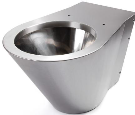
V131 Toilet in stainless steel, for installation against the wall. The V131 has a 102mm diameter outlet and comes with a wall bracket and installation kit. It is practical for environments where high strength and hygiene is required, such as in public toilets, leisure facilities and restaurants. It cannot be dismantled without special tools, making it also suitable for use in high security areas. The toilet seat and installation accessories are not included.
