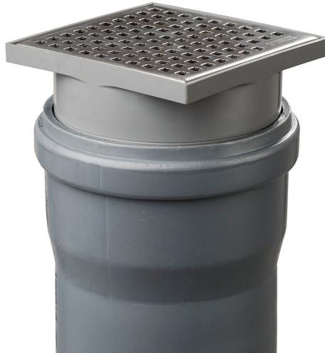
Drain top part that is adjustable and tiltable. Can be mounted directly on to Kvaser and Delling or socket end of a 110 mm waste pipe - enabling installation in areas without need for waterproofing membrane such as concrete flooring
