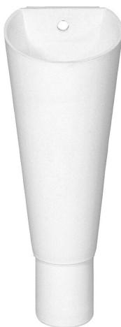
Plastic tundish with rubber seal at one end for insertion of a Ø32 mm outlet pipe. The outlet pipe must be brought up past the gasket and up to the flange of the tundish, in order for the connection between the outlet pipe and the tundish to be smooth.
