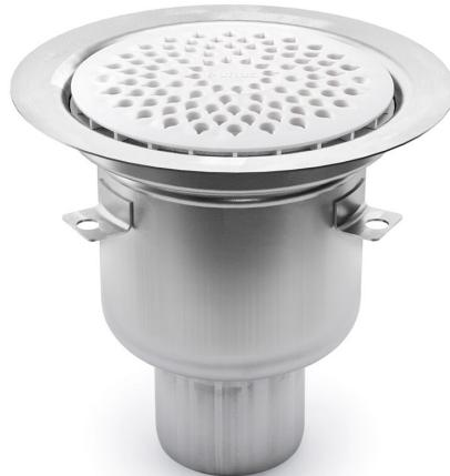
The Balder 75 P untrapped floor drain has a 75 mm vertical outlet and is for installation in wooden or concrete joists. The Balder untrapped floor drain comes with a clamping ring and plastic grate. It also comes with a protective cover that is intended to prevent any concrete or debris from installation from entering the drain.
