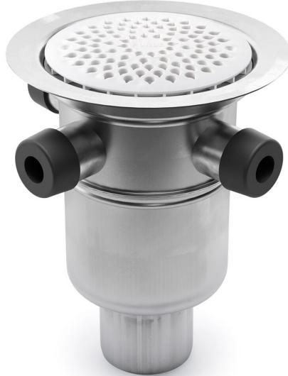
The Baldex 75 P untrapped floor drain has a 75 mm vertical outlet and three extra inlets. Only one of the extra inlets should be used. The gully is suitable for installation in wooden or concrete joists and comes with a clamping ring and plastic grate. It also comes with a protective cover that is intended to prevent any concrete or debris from installation from entering the drain.
