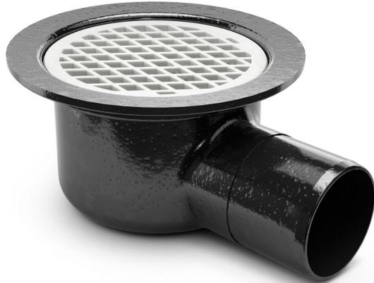
The Bigg 110 E untrapped floor drain is manufactured in epoxy-coated cast iron. It has a 110mm side outlet and can be installed in concrete floors. The Bigg 110 E floor gully comes with a clamping ring and plastic grate, and does not include a water trap. The outlet hole has a protective cover which will prevent any screed or similar from entering the drain.
