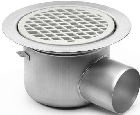
The Bigg 110 P untrapped floor drain has a 110 mm side outlet and is for installation in concrete joists. The Bigg untrapped floor drain comes with a clamping ring and plastic grate. It also comes with a protective cover that is intended to prevent any concrete or debris from installation from entering the drain.
