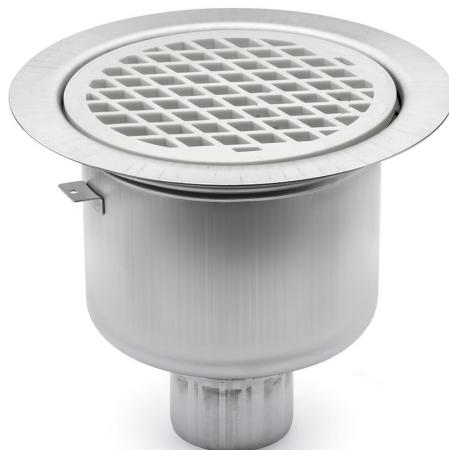
The Heavy 75 P untrapped floor drain has a 75 mm vertical outlet and is for installation in concrete joists. The Heavy untrapped floor drain comes with a clamping ring and plastic grate. It also comes with a protective cover that is intended to prevent any concrete or debris from installation from entering the drain.
