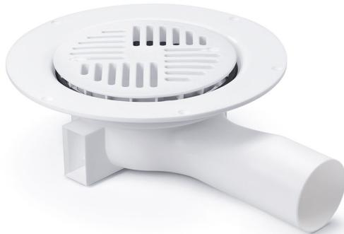
The Minimax 50 Side untrapped floor drain has a 50mm side outlet and is for installation in concrete floors. It has a low construction height of 70mm. The Minimax floor gully comes with a clamping ring and plastic grate, and does not include a water trap. Not suitable for installation underneath a bathtub.
