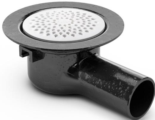
The S/50L MA untrapped floor drain is manufactured in epoxy-coated cast iron. It has a 75mm side outlet and can be installed in concrete or wooden floors. The S/50L MA floor gully comes with a clamping ring and plastic grate, and does not include a water trap. The outlet hole has a protective cover which will prevent any screed or similar from entering the drain.
