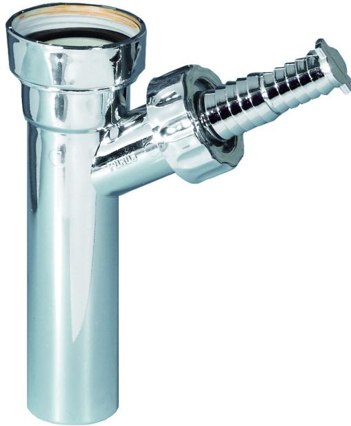
Hose connector 32mm x G32 for dishwashers and washing machines. Includes a G32 wash basin connector. This hose connector is installed within the water lock and replaces the telescopic pipe. The hose connector is suitable for a 15/17/20mm diameter hose.
