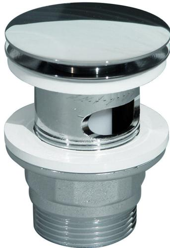
The 1¼" Pop-up waste outlet is a vertical valve for baths. It is manufactured in chrome-plated brass and has a G32 connection. The lid of the valve opens and closes by applying pressure. It also includes a connection for the overflow.
