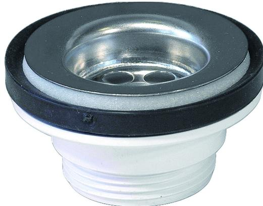
This waste outlet is a plastic vertical outlet for wash basins with a G32 connection. The waste outlet comes with a stainless steel strainer and does not have a connection for an overflow.
