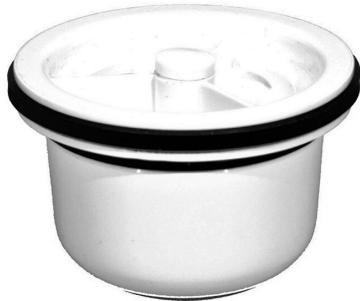
Plastic water trap for shower wastes. The water trap is a mechanical odour stop designed to close when there is no water flow, thus preventing odours from escaping through the drain, even when dried out. It is therefore suitable for environments which have little or no water supply for longer periods of time. When water is flowing through, the water trap opens automatically. It can be removed from the outlet gully for easy cleaning and maintenance.
