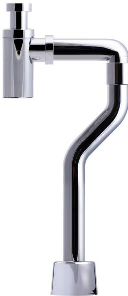
S-Bend water trap kit in chromed plastic, designed for floor connection with a 1 1/4" bottle trap and a 40mm diameter outlet pipe. This water trap kit allows for floor installation directly below the vertical waste, and 320mm to the side. Comes with floor cover.
