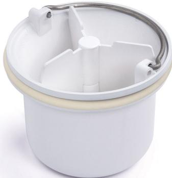
Plastic Flexi-NOOD water trap for Purus' Mini Brage floor gullies. The NOOD no-odour water trap is a mechanical odour stop designed to close when there is no water flow, thus preventing odours from escaping through the drain, even when dried out. It is therefore suitable for environments which have little or no water supply for longer periods of time. When water is flowing through, the water trap opens automatically. It can be removed from the outlet gully for easy cleaning and maintenance.
