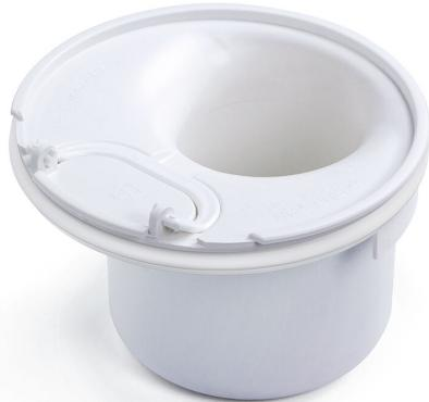
The Ran is a plastic water trap designed for use with most of Purus' 150mm diameter floor gullies. It comes with a rubber seal and plastic handle, and can be removed from the drain for easy cleaning and maintenance.
